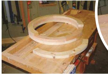
▲ Pic.6 Cut and mitre oversized segments for the final layer, using the frame as a base
